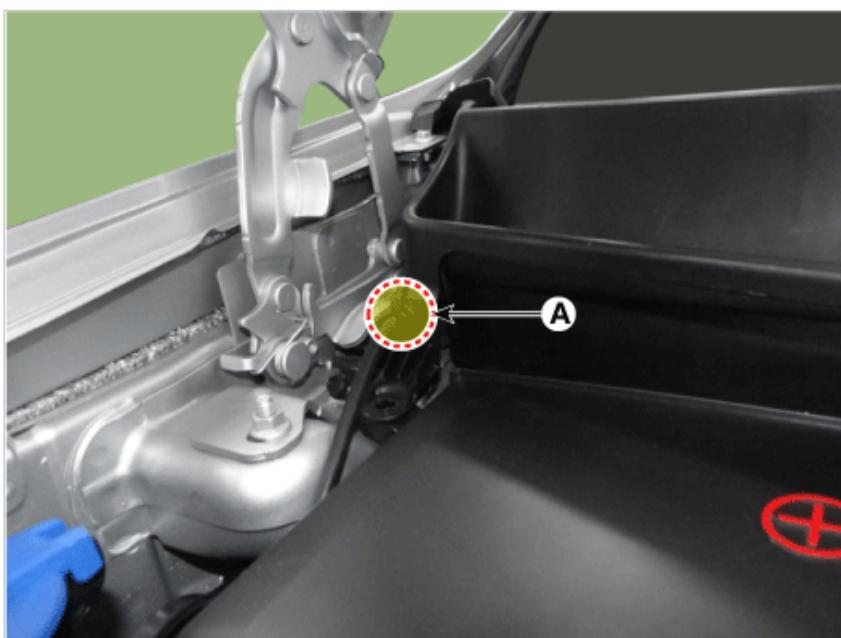
5. Detach the clips, then remove the cowl top cover (A).
